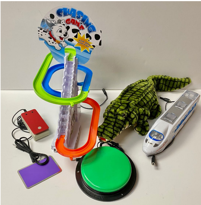
Image 1: Touch switches with switch adapted spotty dog slide toy, alligator and bump and go train.
